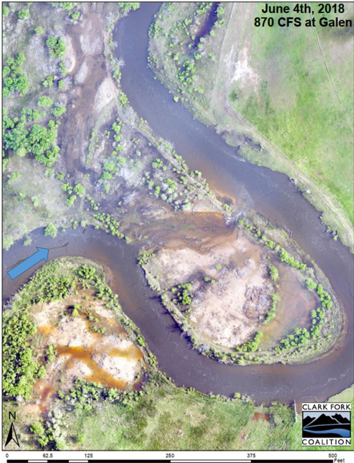
Figure 10- Aerial imagery of a contaminated meander tab in in Phase 3A. Active avulsion pathways are clearly noted with deltaic slicken sediments clearly present at the outlet of the avulsion.
