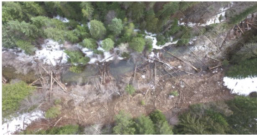
Cedar Creek Road removed and Large Wood Structures Constructed with floodplain connection—2020
